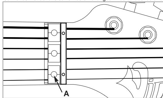
1) Start by loosening screw "A" on the diagram with the 2.5mm Allen key located behind the headstock. Please note: It is not necessary to completely loosen the screw to change your strings.
