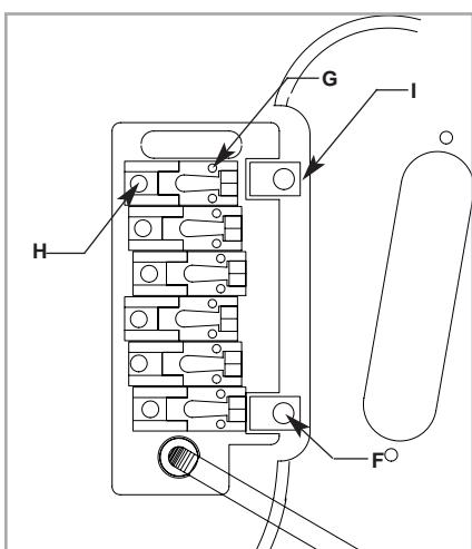
1) Screw "F" adjusts the overall height of the bridge. Before using it, make sure to loosen by 1/10 of turn screw "I".
