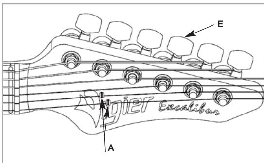
1) Start by loosening the wheel located behind the machineheads. Remove your old set of strings from the rear side of the guitar.
